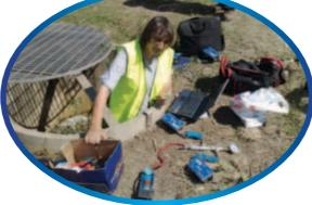
In particular, the deployment and use of equipment such as pressure dataloggers, ultrasonic flowmeters and insertion flowmeters allows NRW Specialists to acquire actual field data on which to base its conclusions and understandings of water supply asset performance. Such information is invaluable when used as an input into network modelling activities and takes the "guesswork" out of the analysis.
